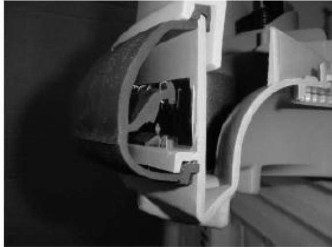
Fig 1.6.1.1. Front bumper cross section
