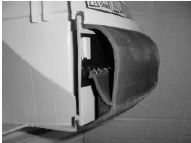
Fig 1.6.2.1. Rear bumper cross section
